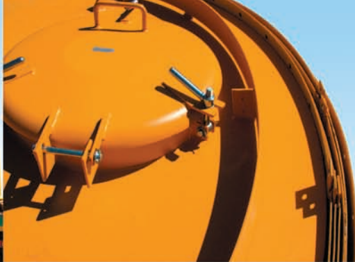
The segments of the silos are piled into one another in order to save space.
